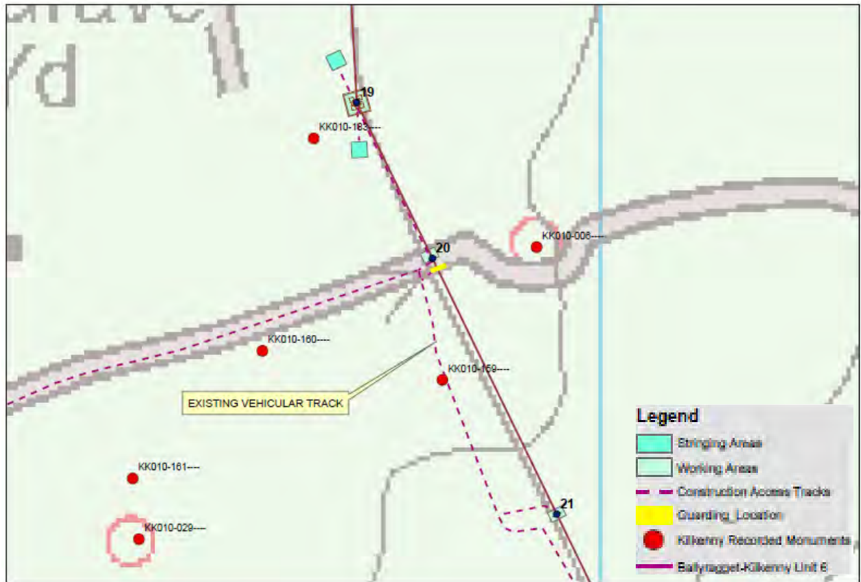
Figure 7.45 Proposed construction access tracks and stringing areas in vicinity of Recorded Monuments
