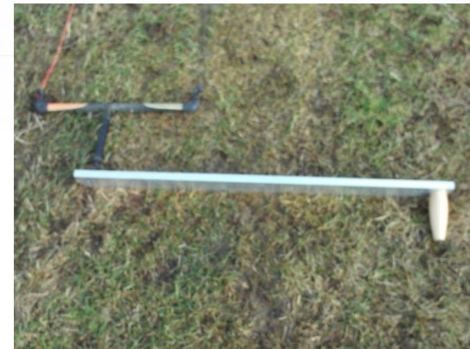
De Prony Brake method: the user retains the lever, the dynamometer showing the strength.
