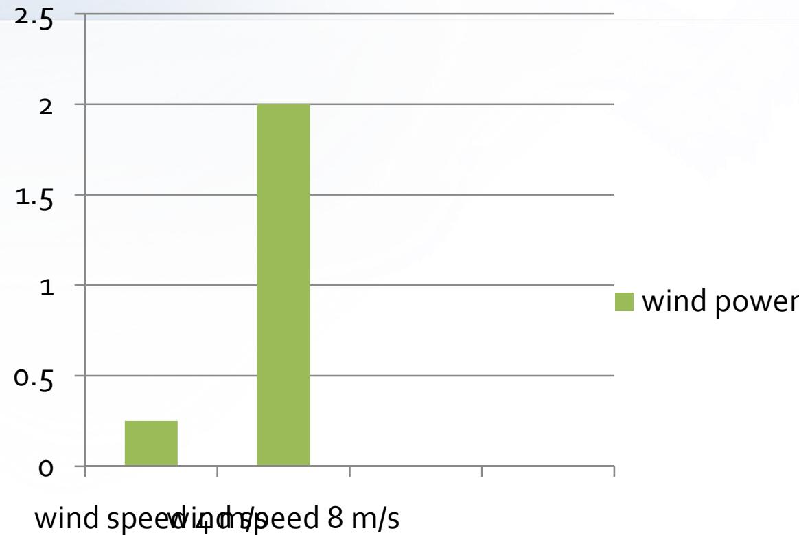
The wind power grows with the cube of its velocity. Wind velocity grows with altitude. At 80 m from the ground the average wind velocity is about 4,6 m/s, and at 1200 m it is about 9,2 m/s.
