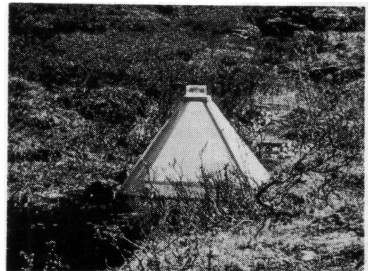
Fig. 3. Emergence traps used in the sampling.
