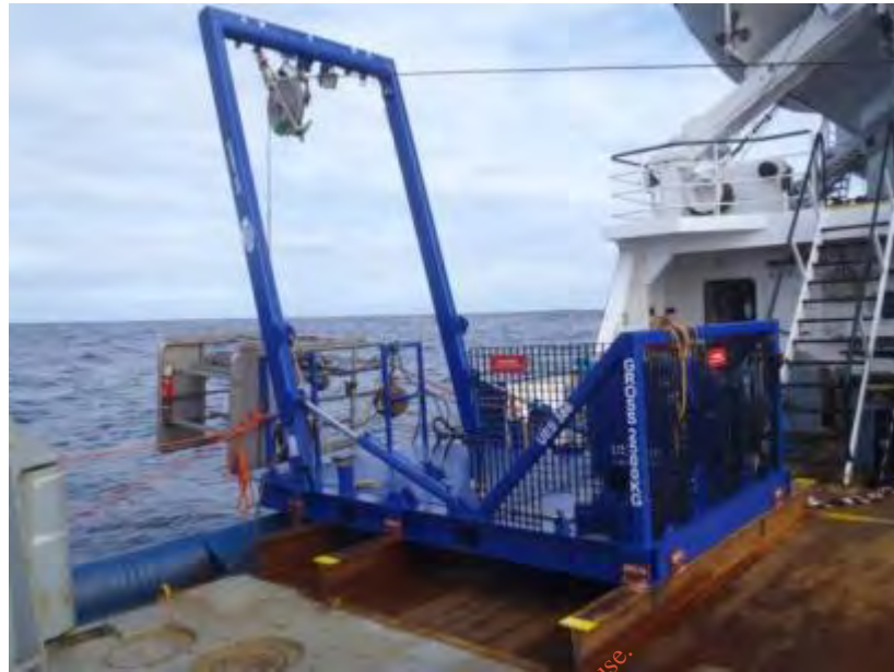
Figure 2.3: Deck LARS system used during the 2014 environmental survey
