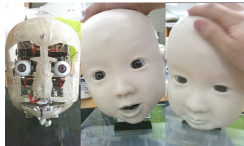
Fig. 1. Internal mechanical structure and appearance of Affetto’s head
