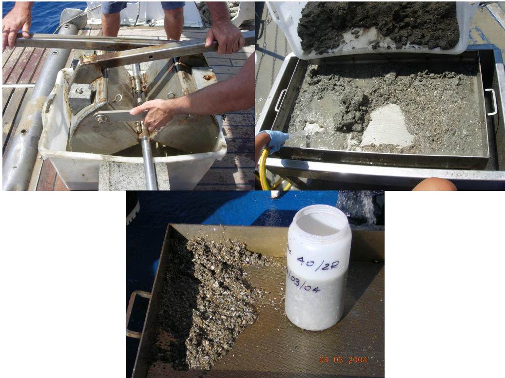
Figure 2.3.2 – Different phases of macrozoobenthos sampling: on board sediment sampled was sieved by 1-mm mesh and preserved in seawater adding 4% CaCO 3 -buffered formalin.
