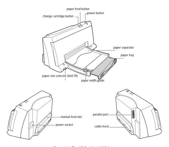
Figure 1-1. The HP DeskJet 400 Printer
