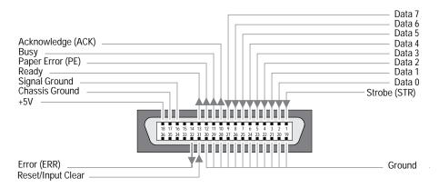
Figure 2-2. Centronics Parallel Interface Connector
