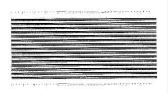
If there are streaks in the horizontal bars or gaps in the diagonal test pattern at the **bottom** of the page, some of the ink nozzles may still be clogged. If necessary, repeat the cleaning process. If the cleaning routine still does not restore the print cartridge, try doing the procedure "Cleaning the Electrical Contacts" later in this chapter.
