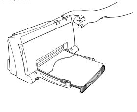
**5.** If the printer has a carriage stall error condition, look for obstructions or binding along the printer carriage path. Slide the print cartridge cradle back and forth across the printer mechanism. If the problem cannot be resolved, return the printer for repair.
