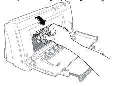
5. Gently remove the tape(s) covering the ink nozzles. Be careful not to touch the ink nozzles or the copper contacts.
