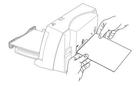
The Paper Feed light will blink when the printer is ready for another sheet of paper.
