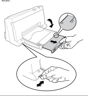
**3**. Insert a stack of paper into the paper tray with the print side down. If you are loading letterheads or HP transparencies, insert them print side down, with the top of the page going into the printer.
