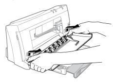
**3.** Open the paper separator (the flap that separates the printed pages from the blank sheets) by pulling it toward you.
