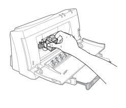
2. Remove the print cartridge from the printer and clean the print cartridge and print cartridge cradle contacts. Use a cotton swab lightly moistened with water. Do not wipe the ink nozzles on the print cartridge.
