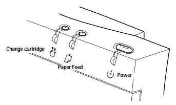
Figure 5-3. Printer Buttons and Lights
