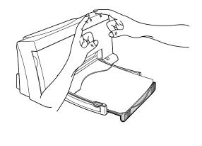
4. If using the printer manually, load a sheet when the Paper Feed light starts blinking. See "Loading Media" in chapter 3 for instructions on manually loading paper.
