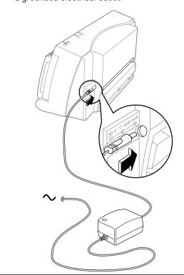
2. If the electrical outlet is on the same side as the parallel port on the printer, fit the power cable into the cable track so that the power cable is neatly housed in place.
