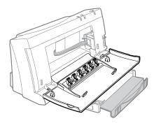
**4.** Turn the printer off. Because of the stall condition, the printer should turn off with the print cartridge out of the home position.
