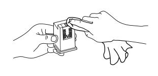
7. Repeat the above steps of installing the print cartridge, cleaning the print cartridge contacts, cleaning the print cartridge cradle contacts, and clearing the nozzles several times. If the problem consistently appears in the printer self-test with the same rows of dots missing on different print cartridges, return the printer for repair.
