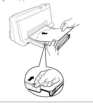
If you are using legal, executive, B5 size paper, envelopes, labels and thick paper, you will have to feed these into the printer manually, one by one . See the section on "Manual Single Load".
