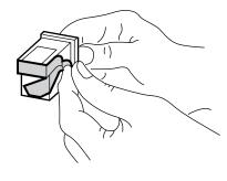
**6.** Insert the print cartridge into the holder at an angle such that the green top is tilted toward you. The arrow on the print cartridge should be pointing toward the inside of the printer.
