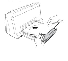
4. Move the paper width guide so that it presses lightly against the paper stack.
