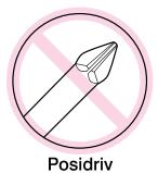
Figure 6-1 Phillips vs. Posidriv Screwdrivers
