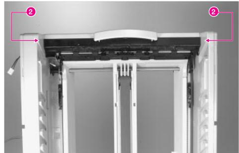
Figure 6-59 Mailbox with Stapler, Flipper Assembly Mounting Screws
