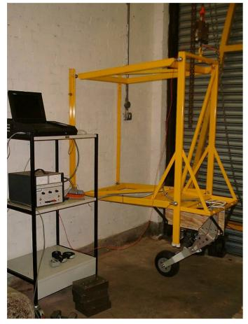
Landing Gear Drop Tests
