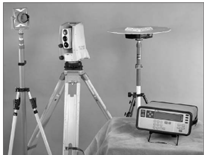
Figure D-2 Trimble 4000 GPS dual frequency receiver with "pizza dish" antenna and TTS 500 total station.
