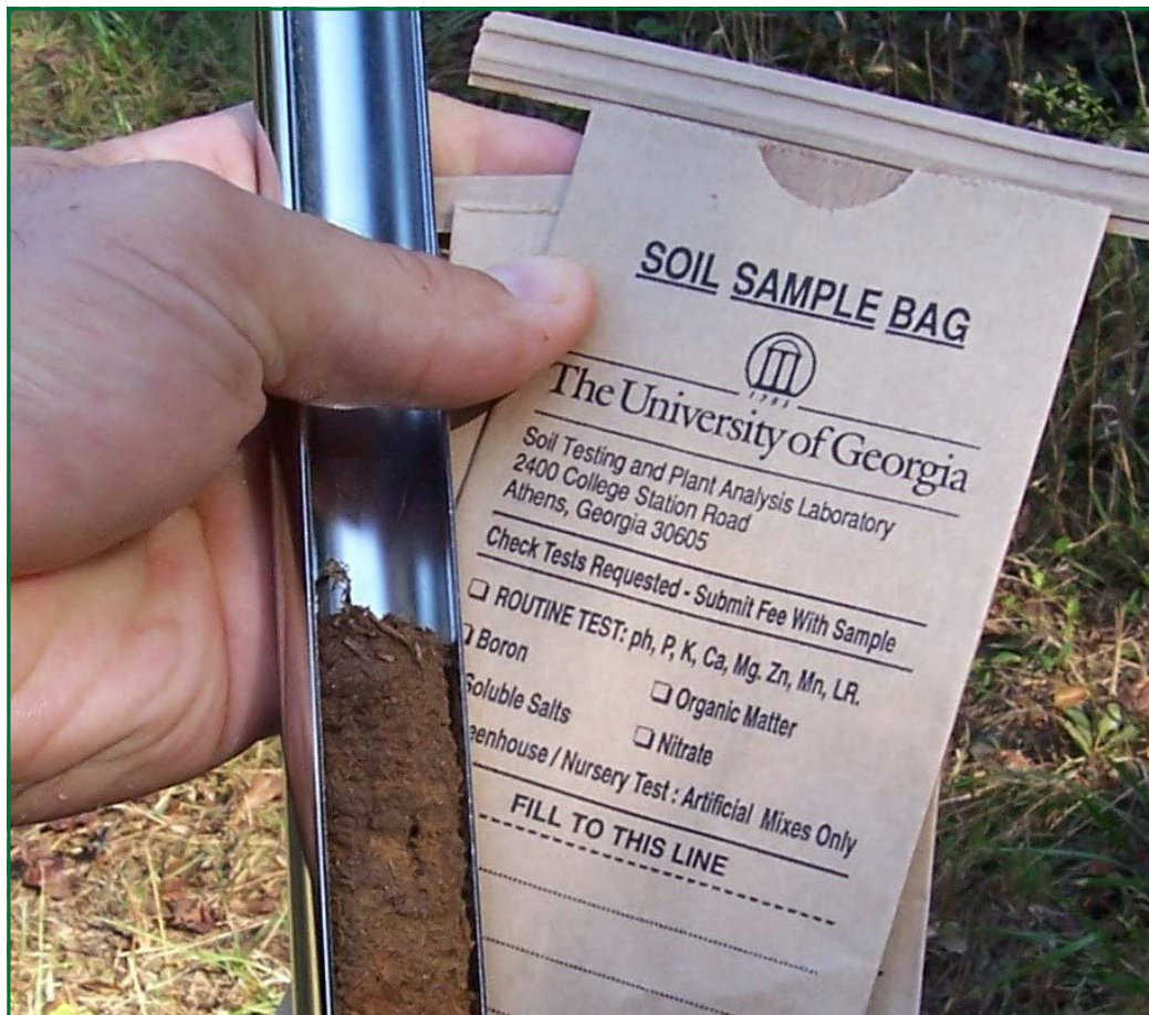
Understanding your soil composition is the first step to fostering an optimal soil ecosystem. A basic soil test measures the level of organic matter, pH, and macronutrients — nitrogen (N), phosphorus (P) and potassium (K). (Special Photo/UGA-CAES)
