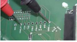
Figure 6-3 Check points for Option CAN-bus
