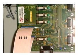
socket J6 on the Optibo board (on the left side).
