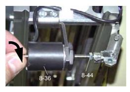
Figure 6-86 Rocker adjustment
