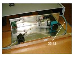
Figure 6-38 Fast wash pump assembly removal
