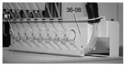
Figure 6-45 Removal of the pinch valve
