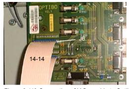
10 Connect the X-flat cable to socket J6 on the Optibo board.
