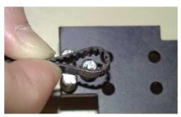
Figure 6-160 Installation of the Y-belt
