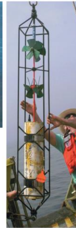
(b) A propeller-type flow meter being brought back aboard a research vessel.
