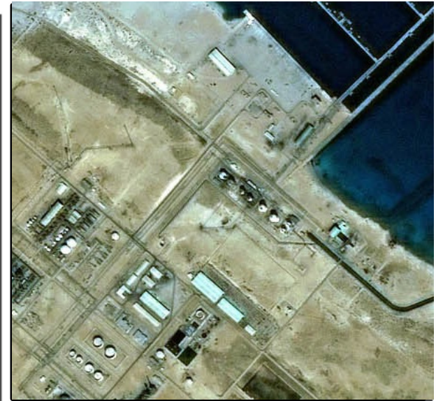
Landsat TM7 & Spot5 Processing LSTM7 MS 30m Pan Sharpened with Spot5 Pan 5m Final Image Resolution 5m
