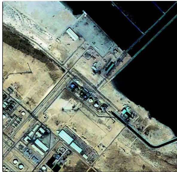
Landsat TM7 & Spot5 Processing LSTM7 MS 30m Fused with Spot5 Pan 5m Final Image Resolution 5m
