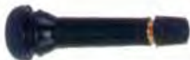
Tubeless valve Type TR418. Fits 11.5mm hole. Length 61.5mm. Complete with caps. 25 per pack TY127
