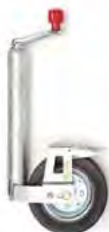
AL-KO Premium jockey wheel 48mm Incorporates weight gauge. Maximum dynamic load bearing capacity 300kg with static capacity 180kg. Tube diameter 48mm with a grooved rubber wheel (230 x 80mm). Boxed 007193B
