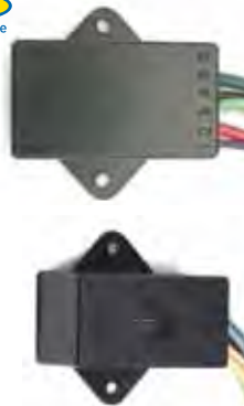
Ring relays Combination Split charge relay for charging auxiliary battery & operating a refrigerator whilst towing. With automatic cut off 014405
