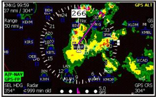
Fig. 3-5 XM Weather - IFR Conditions
