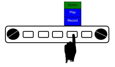
To stop the recording locate the DEMO button and press STOP. Be absolutely certain that a memory stick is in a DU prior to pressing STOP. Data is written to internal memory during the flight, and is transferred to the memory stick when STOP is pressed.
