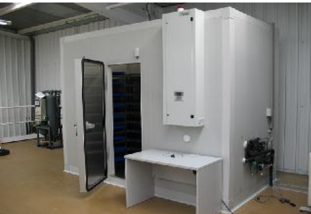
FitoClima 10.000 PH – Pharmaceutical products stability testing
