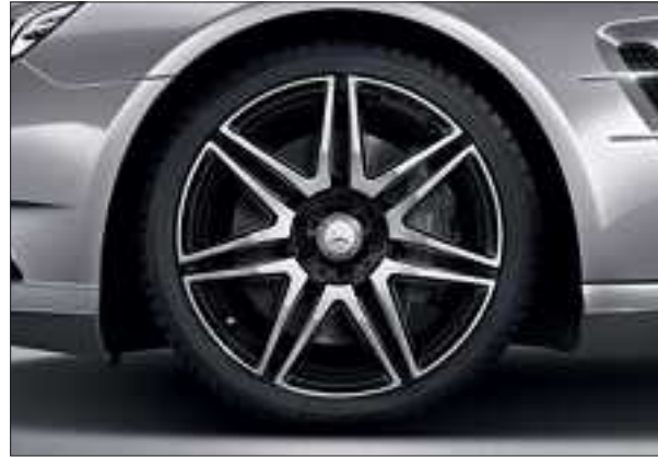
AMG 7-twin-spoke light-alloy wheels in a high-gloss black finish, with 255/35 R 19 front tyres and 285/30 R 19 rear tyres (option, part of the AMG Line, Code 662).
