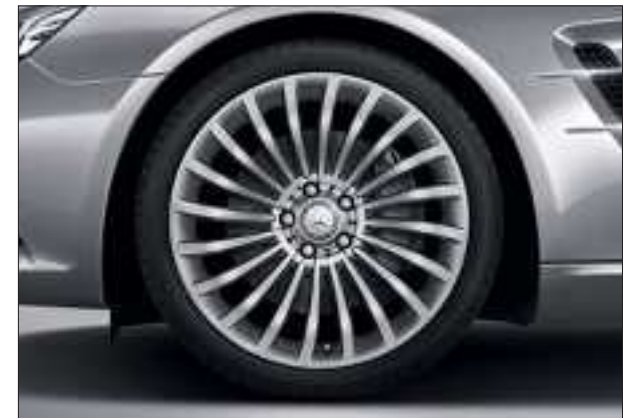
Multi-spoke light-alloy wheels with 255/35 R 19 front tyres and 285/30 R 19 rear tyres optionally available for the rear (ex-factory accessory wheel, Code 11R).
