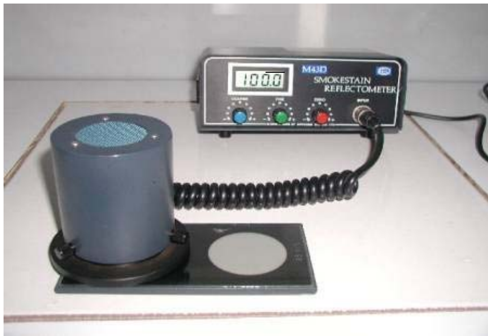
Fig.3.13. EEL Smoke stain reflectometer (Model 43D) for quantification of BC in PM
