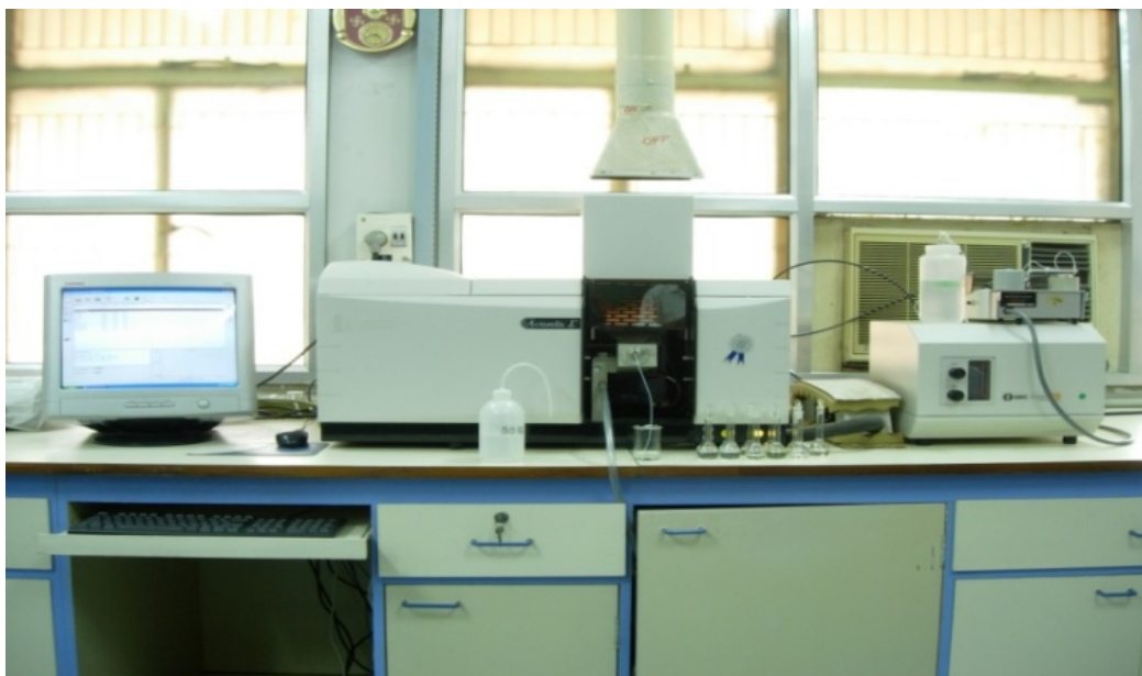
Fig.3.5. Picture of a flame atomic absorption spectrometer (GBC make, model Avanta- \Sigma )
