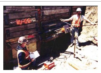
Anchor Tension Load Test in Minneapolis, MN Figure B-2
