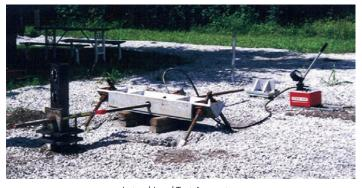
Lateral Load Test Apparatus Figure B-6
