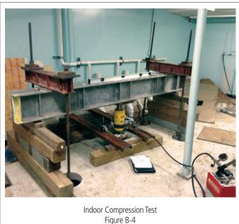
digital gauges (must be accurate to .001") mounted on an independent reference beam, a transit level surveying system, or other types of devices as may be specified by the engineer.
