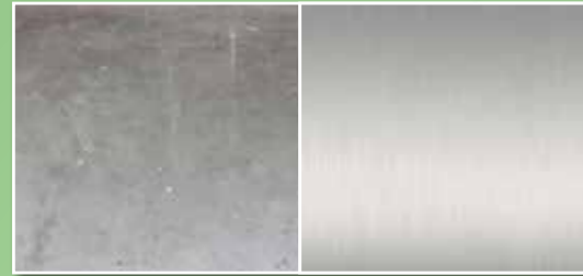
Stainless steel, before and after cleaning
