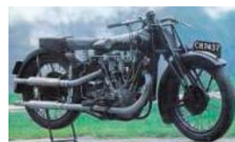
1928 McEvoy 1,000cc v-twin, powered by JAP's legendary 'KTOR' racing engine. Estimate: £28,000 - 34,000
