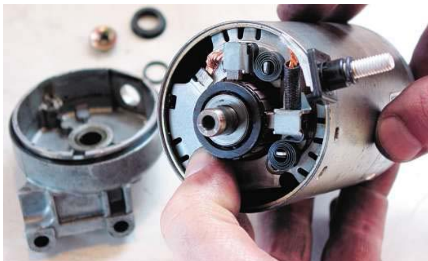
Carbon brushes must be in good condition for the starter to work properly.
