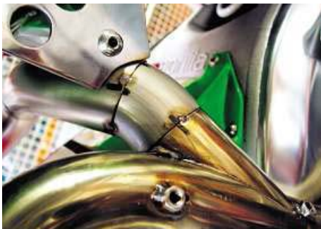
Artistry in metal. These pipe sections are carefully hand cut and welded to make a one-off exhaust system at the Motad factory.
