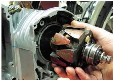
22: At the right-hand side of the engine now, I can refit the generator rotor. This simply clamps up onto a taper on the crank, and one tip I have picked up over the years is to lap the tapers together with a little grinding paste before assembly. Kawasaki triples, in particular, used to shear Woodruff keys as the rotor came loose on its taper. The secret is that the key only locates the rotor in position; the integrity of the taper surface is the bit that actually transfers the load. The GT750 rotor can fit in any position, and doesn't use a key.
