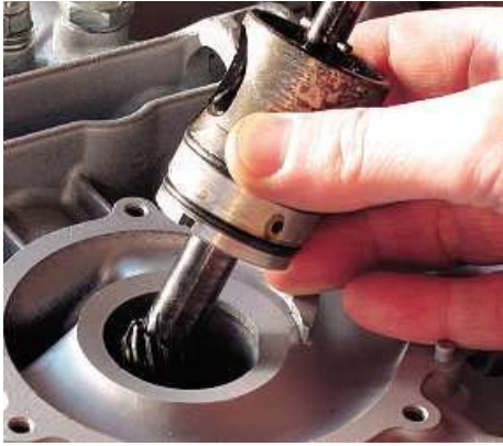
18: Next, the water pump. I've turned the bottom end upside down on the bench to make the pump body easier to fit, and made sure it's turning freely before offering it into the crankcase. Again, note the O-rings that act as seals on the pump body. The body is notched, and will only fit the correct way. Once it's fully home a circlip secures it in place.
