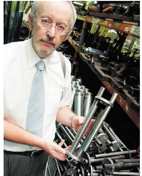
Motad's Rob Limbrick demonstrates the internal baffle assemblies used in traditional silencers for road use.
