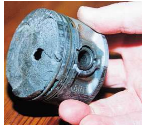
Number three piston, terminally damaged by the effects of detonation.
