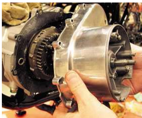
25: Now the inner timing cover can be fitted over the starter clutch and clamped up to its new gasket. This may look like a complex set-up, but in service the whole ignition system can be removed as an assembly and laid aside without disturbing the timing, useful if rapid access is required to the starter clutch or water pump drive gear. I bet it was a boon at the trackside in the Kettle's racing heyday.
