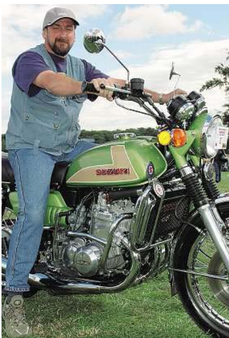
Philip Ryan's GT750 is a tastefully assembled hybrid of early GT750K mated to a twin disc front end.
