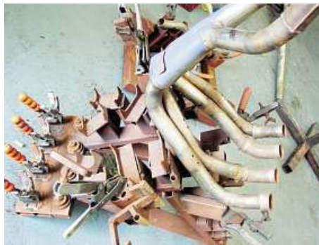
For production, jigs are made for each system to clamp everything up squarely before welding.
