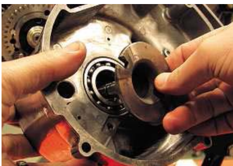
24: At the other side of the engine I'm going to fit the inner timing cover. Firstly this short drive shaft has to be located correctly in its bearing in the cover. This shaft drives the ignition system, so it must be keyed to the crank. The notch you can see at the top locates with a peg on the starter clutch, and be aware that the shaft and starter clutch must be a matching pair. Some shafts had the drive notch in a different position, and if you mix and match them you may have serious problems timing the ignition.
