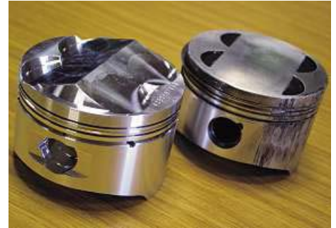
The replacement pistons from Wiseco have much higher crowns for an increased compression ratio.
