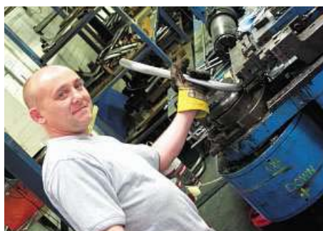
Despite specialised CNC pipe bending machinery, a lot of good old-fashioned skill still goes into making exhaust headers.
