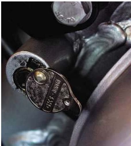
Remove your steering lock before having the frame powder coated.
