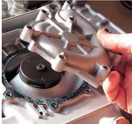
19: Again, I've checked to make sure everything rotates correctly before proceeding; as the crank is turned over the water pump shaft should now rotate. Next I can fit the impeller to the end of the water pump shaft and secure it with a circlip, before fitting the impeller housing with a new gasket.
