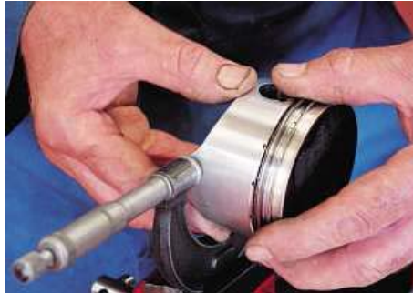
Jim Morley at JME Engineering carefully measured all the pistons before concluding the bores were too tight.
