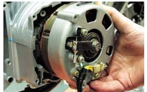
23: Roy has located a brand-new generator stator, which takes the sweat out of cleaning up the old one. This slots over the rotor and bolts up to the crankcase with three long screws. Note the piece of wire protruding from the brush holder, this is holding the brushes back in their holder to make the stator easier to fit. Once bolted up I can pull the wire out, and the two brushes will spring outwards to sit on the commutator. The brushes must be in good condition or the bike may not charge correctly – these are, of course, brand-new.
