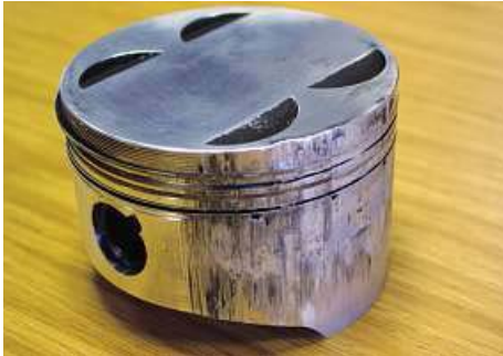
Number three piston after it picked up in the bore at speed on the way to Lotherton Hall.
