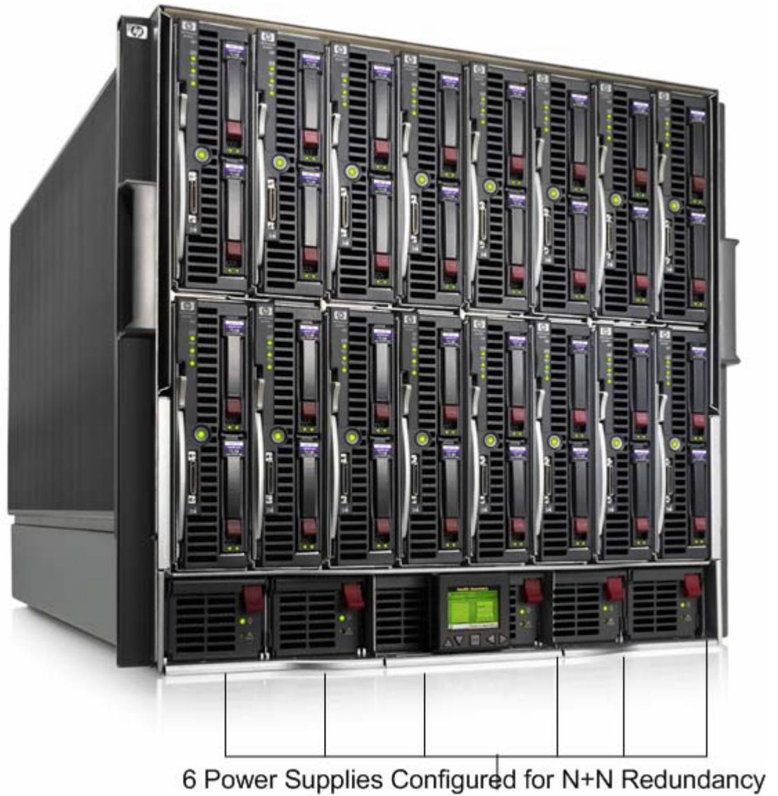
Figure 2. HP c7000 enclosure (front-view) with power configured to run VMware Infrastructure 3 for this reference configuration
