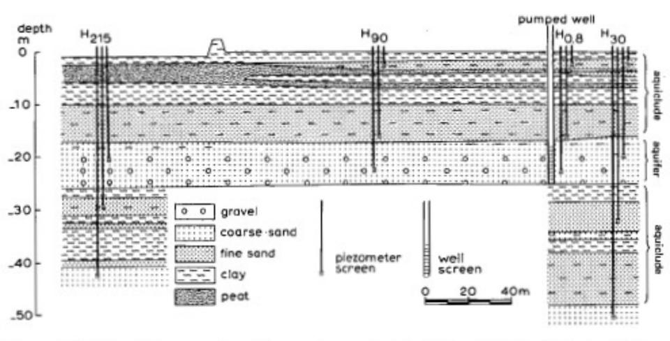
Figure 3.2 Lithological cross-section of the pumping-test site 'Oude Korendijk', The Netherlands (after Wit 1963)
