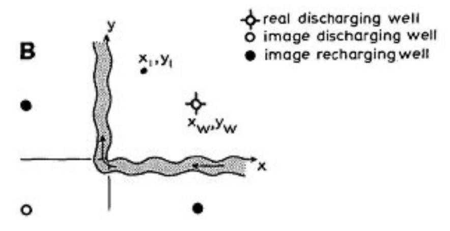
$$G(x,y) = \frac{1}{2} \ln \frac{\left[ (x_1 - x_w)^2 + (y_1 + y_w)^2 \right] \left[ (x_1 + x_w)^2 + (y_1 - y_w)^2 \right]}{\left[ (x_1 - x_w)^2 + (y_1 - y_w)^2 \right] \left[ (x_1 + x_w)^2 + (y_1 + y_w)^2 \right]}$$
