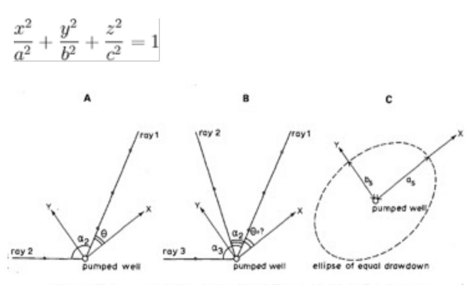
Figure 8.1 The parameters in the Hantush and the Hantush-Thomas methods for aquifers with anisotropy on the horizontal plane:
