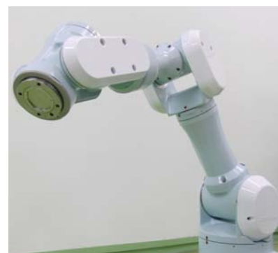
A robot arm with 7 degrees of freedom
