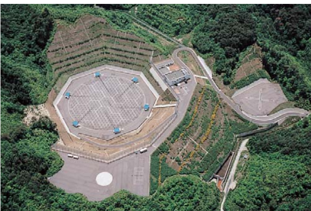
MU radar in Shigaraki, Koka City, Shiga Prefecture. The diameter of the antenna is 103 m.
