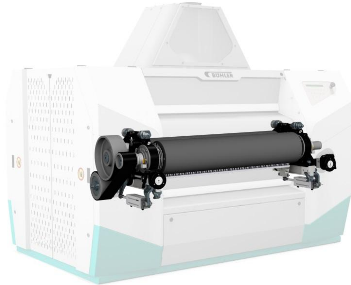
Quick roll change with Roll Quick Pack
