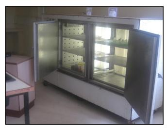
Figure 3. Insect rearing incubator with controlled temperature and humidity
