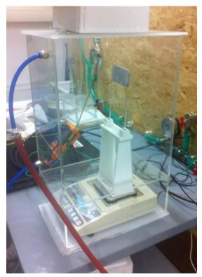
**Figure2.** The whole measuring setup: digital balance, Styrofoam support and the asymmetrical capacitor inside the measuring air-tight chamber.
