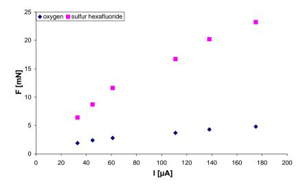
**Figure3.** *Relation between the force* F *generated on the asymmetrical capacitor and the electrical current* I *flowing between the capacitor electrodes for oxygen and sulfur hexafluoride.*
