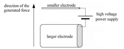
Figure 1. Principle of the force generated on the asymmetrical capacitor.
