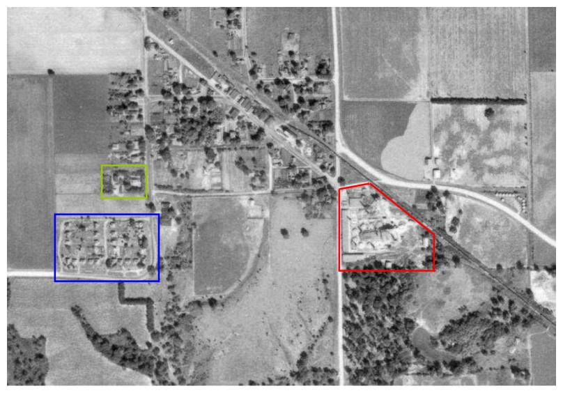
Figure 4. A 1941 aerial photograph of Alsey, Illinois. The Alsey Brick and Tile Company manufacturing plant is outlined in red; the beehive kilns are quite visible. The twenty-two house planned community for the plant workers and their families is outlined in blue. The residence of H. T. McLaughlin, owner of the company from 1911-1959, is outlined in green.
