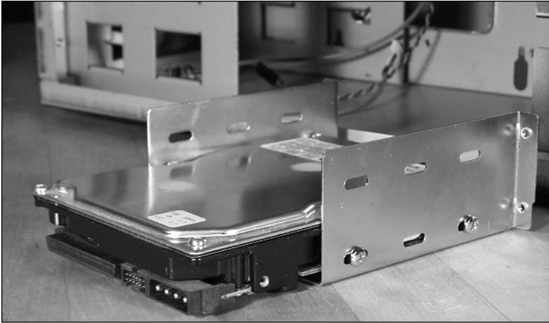
Figure 8-10: Position drives in mounting brackets so they'll get good air flow and heat conduction.
