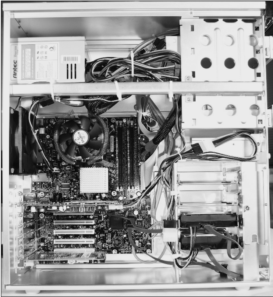
Figure 25-21: Completed system internal view
