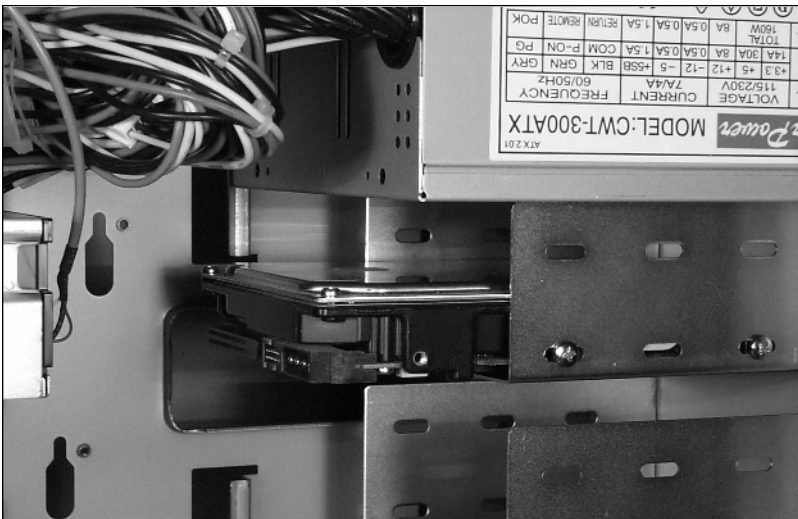
Figure 8-11: Choose positions within mounting brackets to get the best service access within the chassis.
