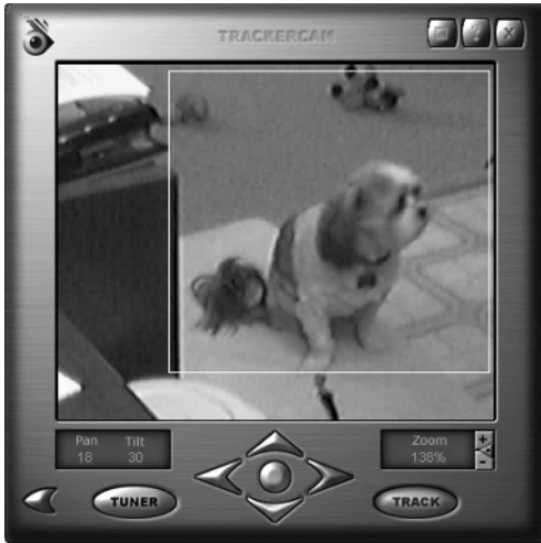
Figure 23-10: A bounding box in the camera view shows the area TrackerCam identified as containing motion.
