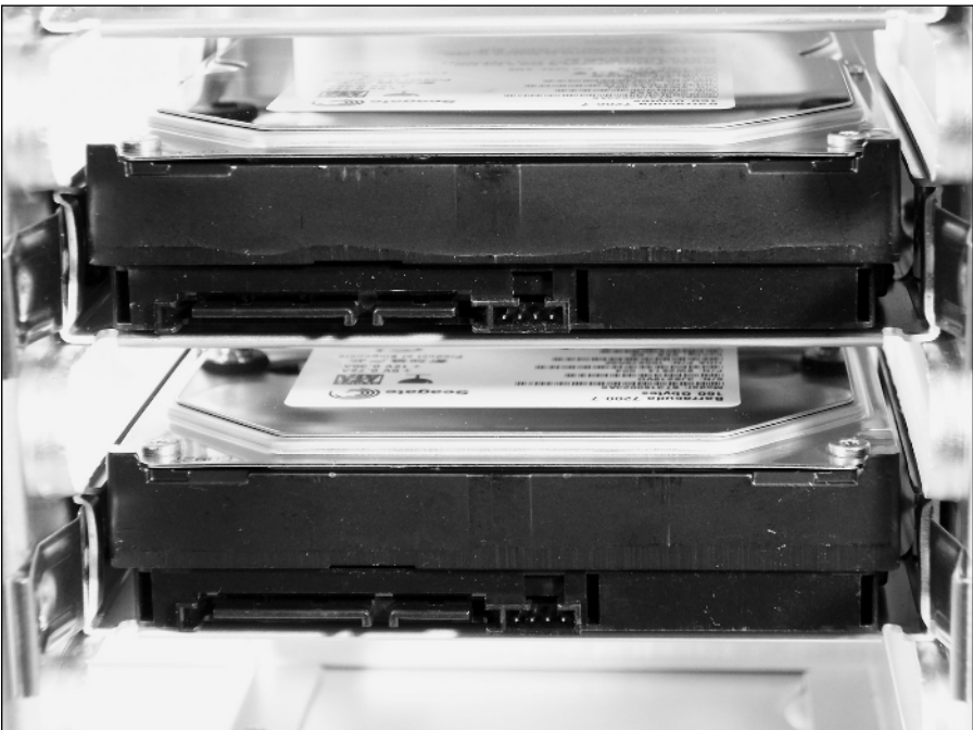
Figure 25-4: Disk drives mounted in chassis
