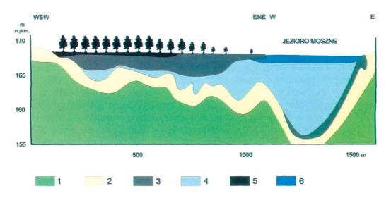
Figure 2. Cross-section of Lake Moszne mire complex. 1 – Cretatious limestone, 2 – glacial and fluvoglacial deposits, 3 – slightly degraded peat, 4 – lake deposits, 5 – degraded peat, 6 – water (from: Harasimiuk, 2009)
