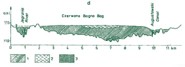
Figure 3. Schematic cross-section of the Red Bog mire in the Biebrza Middle Basin. 1 – sedge and sedge-moss peat; 2 – Sphagnum peat; 3 – gyttja.
