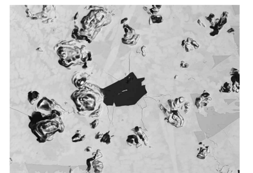
Fig. 8. Peculiar ornate structures in the iron silicide matrix lacking a conclusive explanation. Possibly spotty melting of the matrix.
