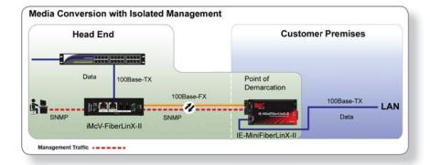
The diagram illustrates a FiberLinX-II deployment with an IE-MiniFiberLinX-II acting as the CPE at the customer demarcation point. The devices are configured so that management data is isolated from customer data, and does not pass through to the customer LAN, while common media conversion functionality is performed without interruption.
