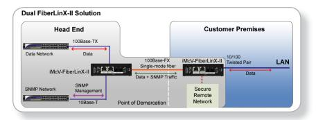
When used in pairs, a FiberLinX-II configured as a Host resides at the head-end while another FiberLinX-II, configured as a Remote, installs at the customer location, typically on the network edge where a customer network meets the service provider infrastructure. Via SNMP, FiberLinX-II monitors the entire link and ensures data integrity while remaining isolated and completely transparent to the customer LAN.
