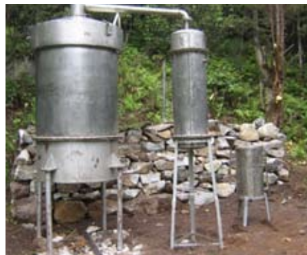
Two types of distillation units: (left) A wet steam distillation unit. (right) A dry steam distillation unit. The DU on the left is made in Nepal and installed in Ghunsa of Kanchenjunga conservation area, whereas the DU on the right is made in India and installed in Syaubari BZCF of Langtang National Park Buffer Zone Area
