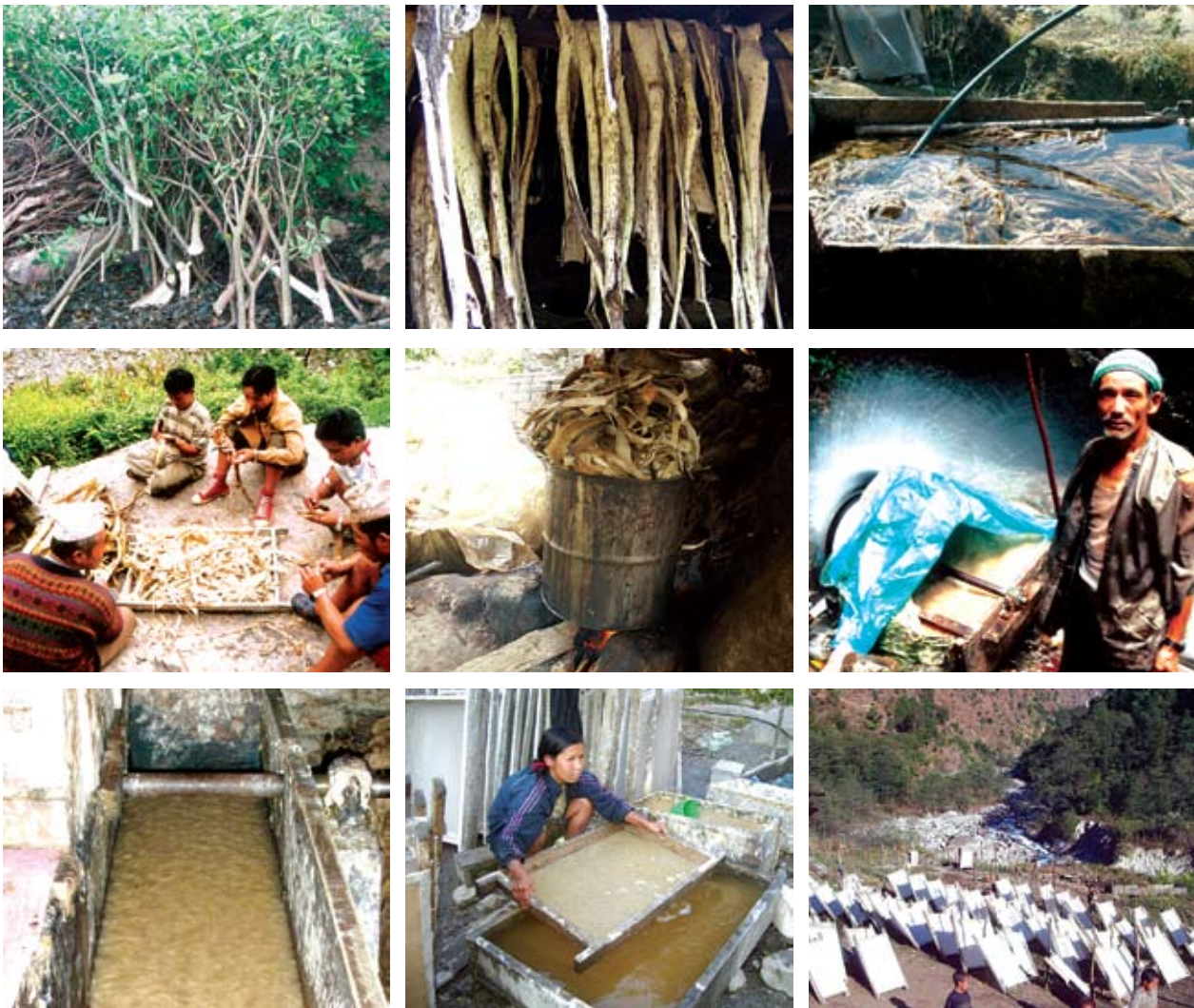
(Top row left to right) Cut stumps of Argeli; Sun-dried bark; Bark soaked in Water for paper making. (Middle row left to right) Cleansing and making small strips of bark; Boiling the bark; Beating the bark with the help of a hydro beater. (Lower row left to right) Beaten bark; Worker making paper; Paper drying in the sun.
