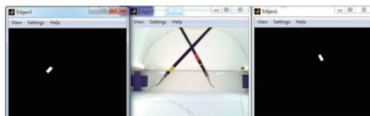
Figure 4. Left: the yellow label's location; Middle: the instruments with label; Right: the red label's location
