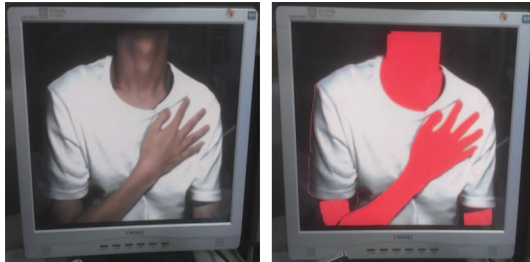
Figure 9. Skin detection result. The Skin part is detected red in the right figure.
