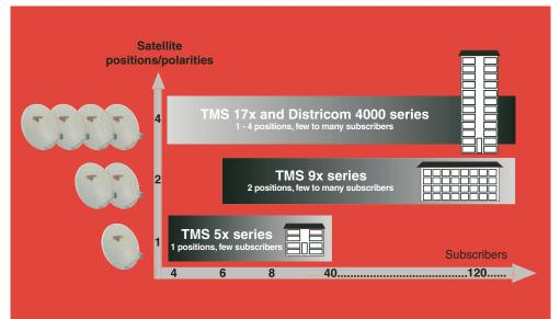
The number of satellite positions/polarities and subscriber outputs is the prime criteria for choosing the right multi switch system.
