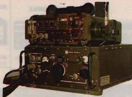
SOUTHCAM SC 130 - Ricetrasmittitore SSB - 2-12 MHz, 20 Watt out, con lineare SC 200A, 200 W out.
