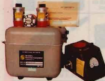
STRUTHERS, RF directional SWR / WATTMETER TS-1285B , with complex detector, CU-753B, CU-754B, CU-755B, and case carrying CY 2606B (new cond.).
