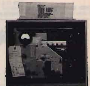
ANALIZZATORE - CAPACIMETRO ZN-3A/U Technical characteristics Leakage volta range: 0-to 600-volt dc; Leakage current range: 0 to 50 ma dc; Insulation resistance range: 1:1 to 100 meg - 110 to 10,000 meg; Capacitance range 0.5 to 100 µf - 80 to 50,000 µf - .04 to 30 µf - 25 to 1,000 µf - 250 to 10,000 µf; Power factor range: 0 to 50 percent. Number of tubes: 9; Power source: Analyzer ZM-3/U: 105 to 125 or 210 to 250 volt ac, 50 to 1,600 cps (cycles per second); Analyzer ZM-3A/U: 105 to 125 or 210 to 250 volt ac, 50 to 1,000 cps.
