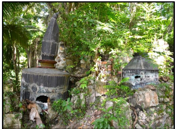
Photo 122. The copper rum stills either side of the second red-brick chimney at the Brewer's Bay Sugar Works.
