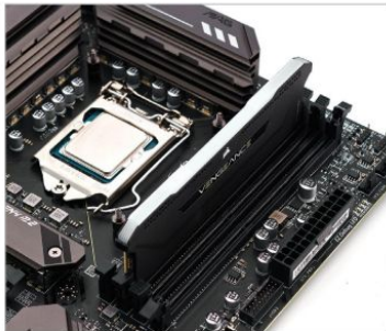
Accompanied by a rewarding click, sticks of RAM are very easy to add to your build.
