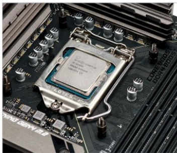
Always make sure the arrows are matching and take your time—CPU pins are super-delicate.
