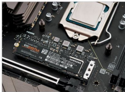
M.2 SSDs are installed directly on to the mobo; undo the little screw, and slot the drive into position.
