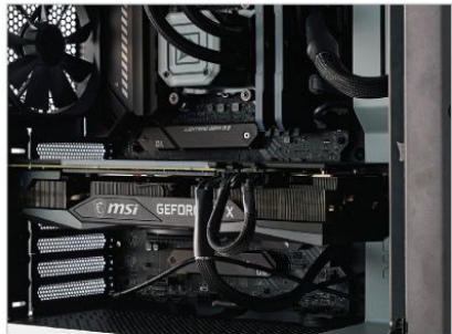
Remove the two PCIe blanking plates from your case before dropping a graphics card into the slot.
