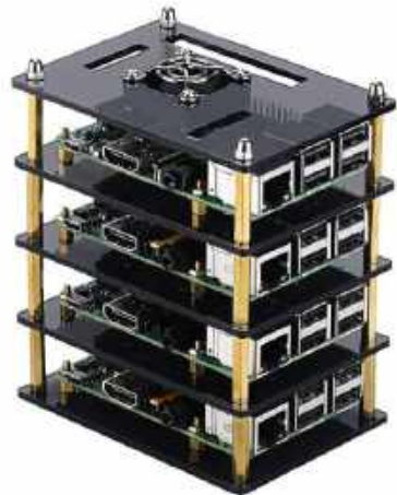
A Raspberry Pi 4 cluster case by MakerFun, with four Pis installed.
