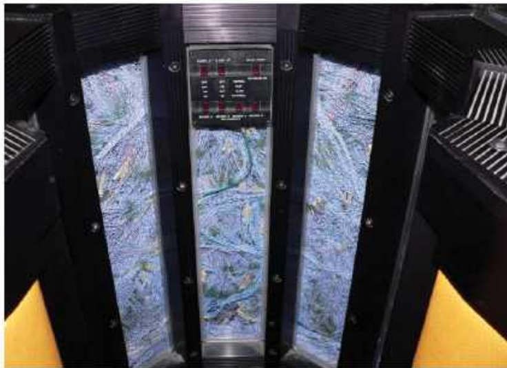
The Cray-2's internal wiring. And you thought your PC cables were a mess!
