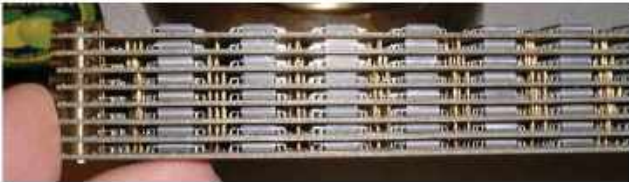
A Cray-2 logic module, showing the tight packing of components
