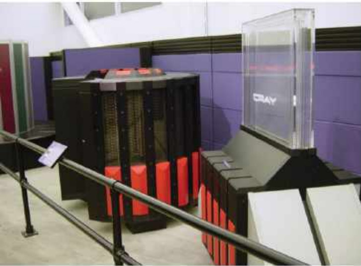
A Cray-2 (left) and its cooling system (right) on display at the computer History Museum
