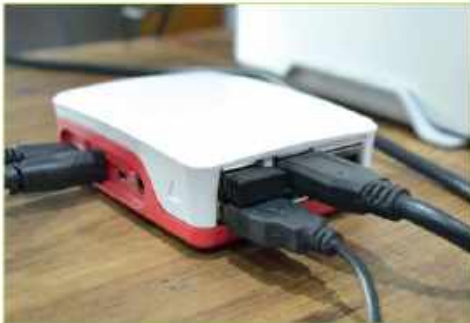
» Connect a USB drive or full-size external hard disk drive to your Raspberry Pi for storage with Nextcloud—USB 3.0 preferred!
