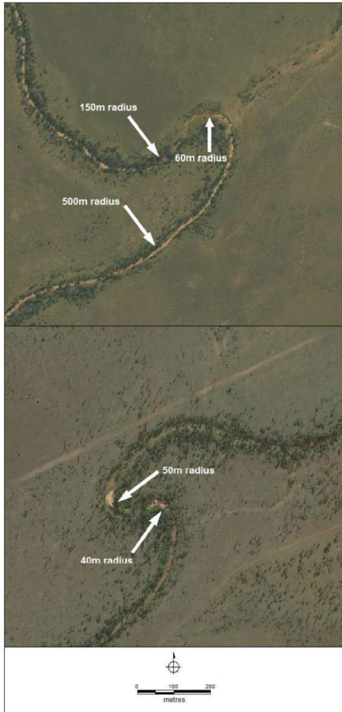
Figure 3.2 - Tight bends at diversion reach and downstream of ML boundary
