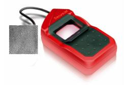
SecureJet Auth-Fingerprint is a sophisticated biometrics sensor allowing users to enroll and authenticate on hp LaserJet MFPs using their finger instead of their login and password.
