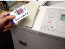
SecureJet Auth-PX is a sophisticated badge reader directly connected to the hp LaserJet MFP motherboard, combined with a software running inside the printer.
