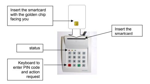
The smartcard must be inserted with the golden contacts facing you. Once the smartcard is inserted, the yellow LED changes from blinking to permanent lit. This indicates the card is waiting for its PIN code.
