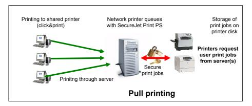
Push printing requires the SecureJet Print SMP module, and Pull printing requires in addition the SecureJet Print PS module on print servers. Authentication can be performed by SecureJet Auth modules or built-in authentication providing the user login name information.
