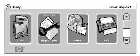
Press the SecureJet button to reclaim your jobs. Authentication is required, using your PIN code or card (depending on the SecureJet product installed).
