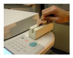
SecureJet Auth-SW is a sophisticated swipe badge reader directly connected to the hp LaserJet printer/MFP motherboard, combined with a software running inside that printer/MFP.
