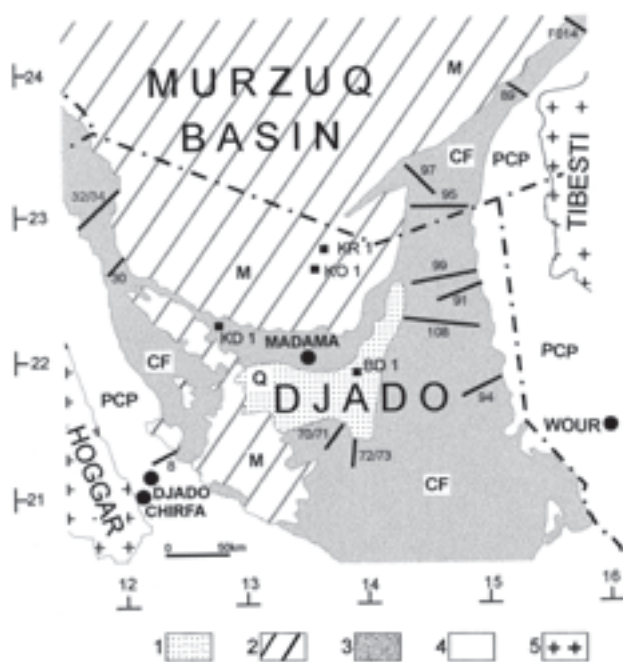
Fig. 1 Simplified geological map of the South Murzuq Basin and Djado sub-basin, with location of geological sections (lines) and boreholes (black rectangles). Explanations: 1 – Quaternary (Q); 2 – Mesozoic (M); 3 – Carboniferous (CF); 4 – Pre-Carboniferous Palaeozoic (PCP); 5 – Precambrian basement.
