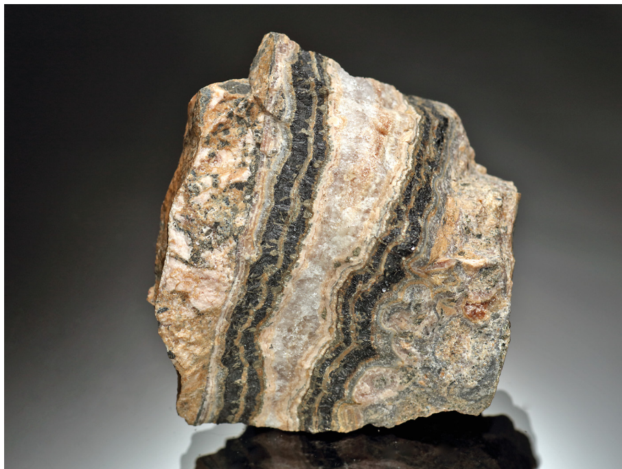
Fig. 1 Ore vein with symmetrically arranged black double bands of cronstedtite. National Museum, Prague, catalog number PIN 111848. Photo P. Škácha.
