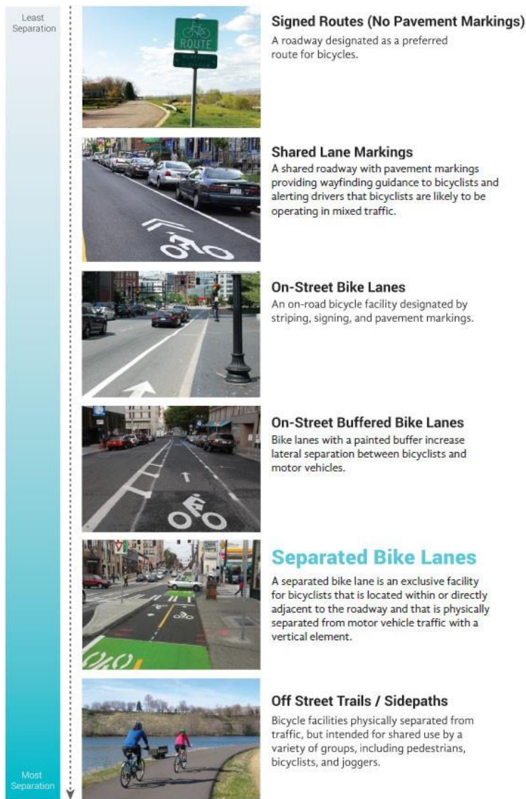
Figure 20. Bicycle Lane Options (Source: FHWA)
