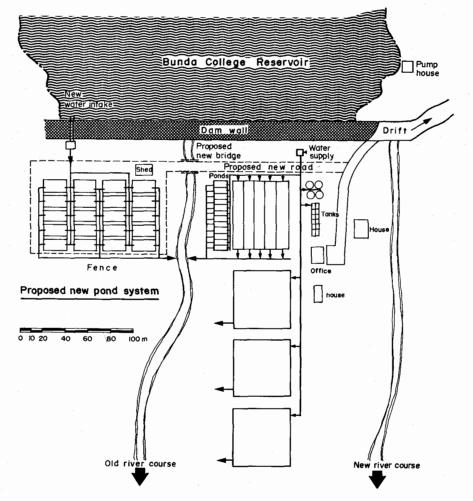
Fig. 7.10. Suggested layout of the ICLARM/GTZ-FD-UM Collaborative Fish Farming Project and 20 x 200 m<sup>2</sup> research ponds at Bunda College of Agriculture, Malaŵi.
