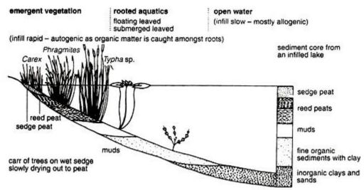
Fig 4.56 : Successional changes in an infilling lake. Illustrated on the right is the core of an old unfilled lake showing the column of sediment (a record of a lakes history)
