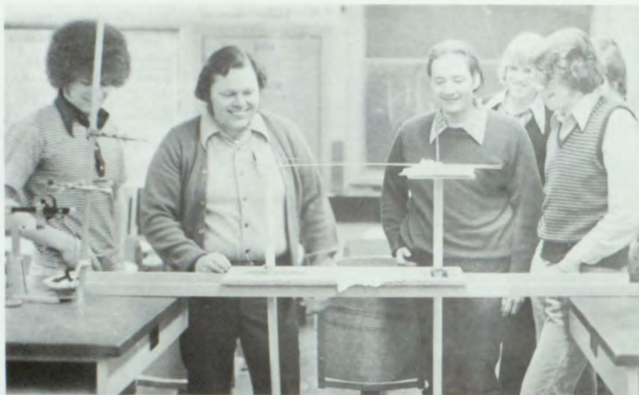
Phil Myerchin demonstrates a 2-dimensional harmonic wave drawing apparatus to his physics class.
