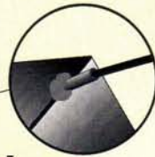
FIG. 5 cross spars insert into end cap fittings
