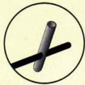
FIG. 2 spar fittings are made by passing vertical spars through vinyl end caps
