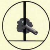
FIG. 3 fittings and vertical spars are glued into place at each corner
