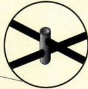
FIG. 4 cross spars are joined by vinyl end caps, pierced at 90-degree angles
